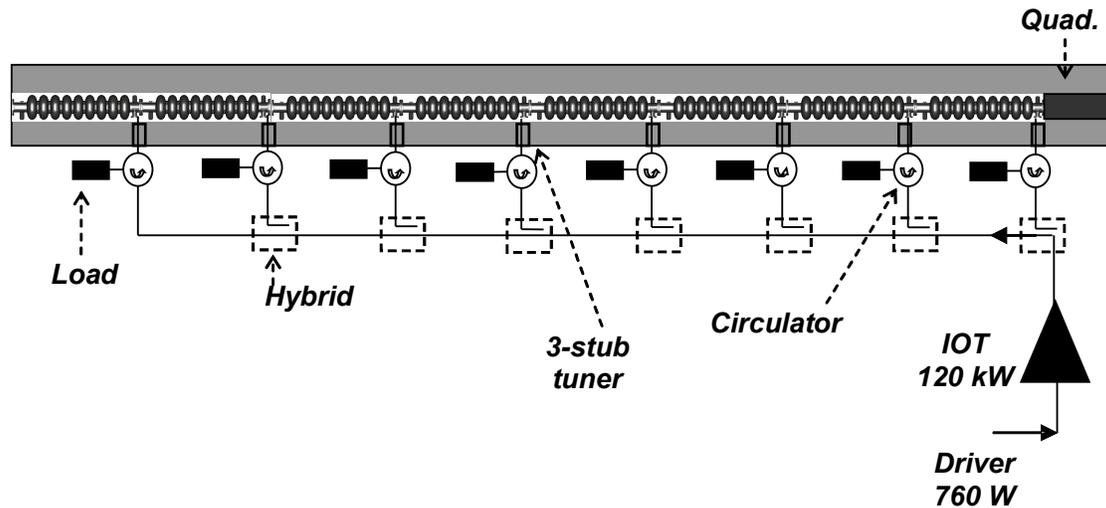
Figure 2: The accelerating unit with the 120 kW IOT, a driving amplifier, a power distribution system and the cryomodule housing eight 9-cell superconducting cavities.
