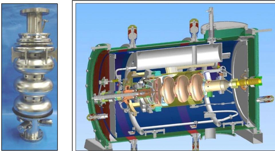
Figure 1. Superconducting cavity of the FZR gun (links) and cross-section of the cryostat (right)
