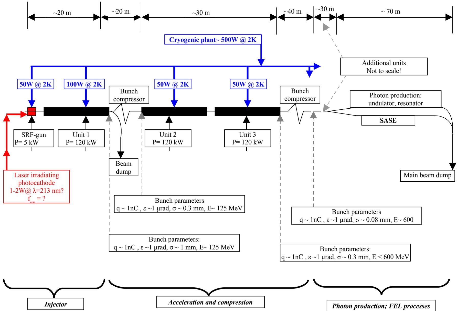
Figure 3: Schematic layout of the FEL facility
