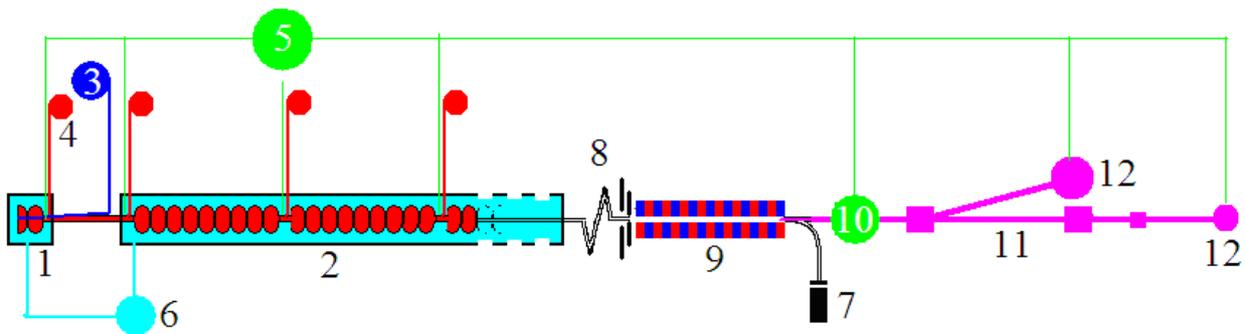
1 – electron injector, 2 – cryomodules, 3 – UV laser activating photocathode, 4 – microwave source (IOT), 5- synchronization and diagnostic system, 6 – cryogenics, 7 – electron beam dump, 8 – electron beam compressor and collimator, 9 – undulator, 10 – photon diagnostics system, 11 photon beamlines, 12 – experimental chambers
